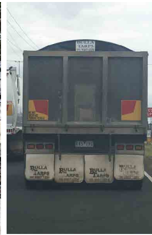
Figure 41 Example of truck tarp that can be used to contain EPS during transport
